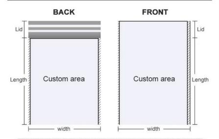
The edge pressing on both sides of the bag is 1cm (diagonal area). Please also pay attention to the design of the drawing. The width of the hot sol is about 1cm.
